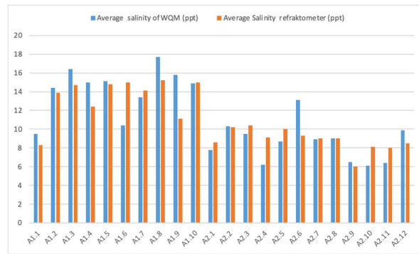
Figure 3. Salinity measurement results of WQM sensors and refraktometer in the first trial
